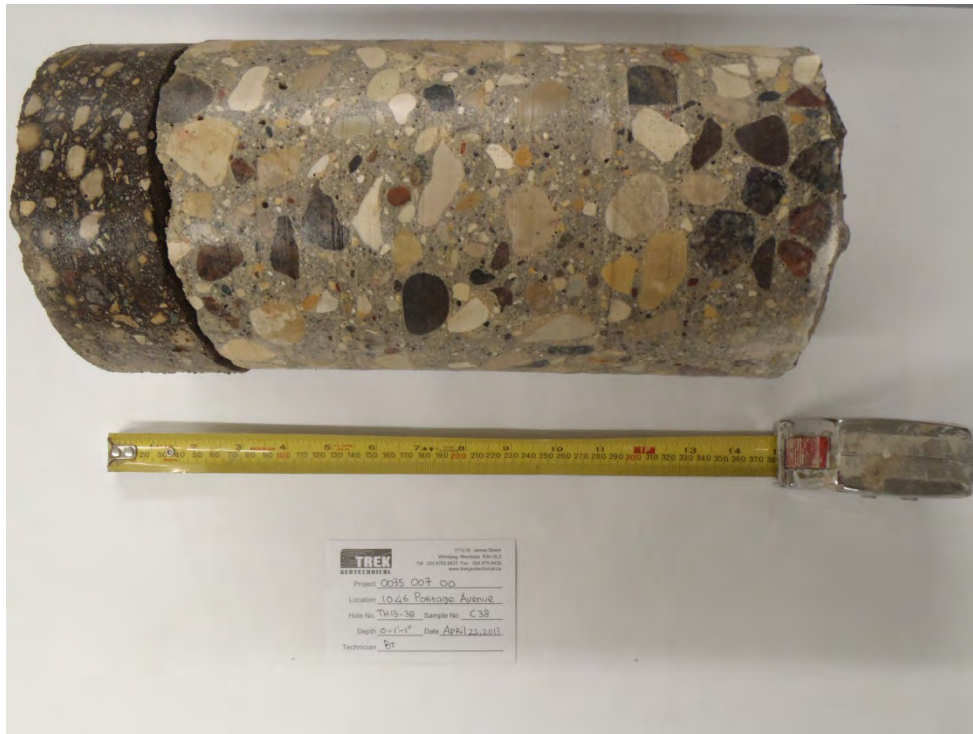
Photo 45: Asphalt and Concrete Core Sample from Test Hole TH13-38B
