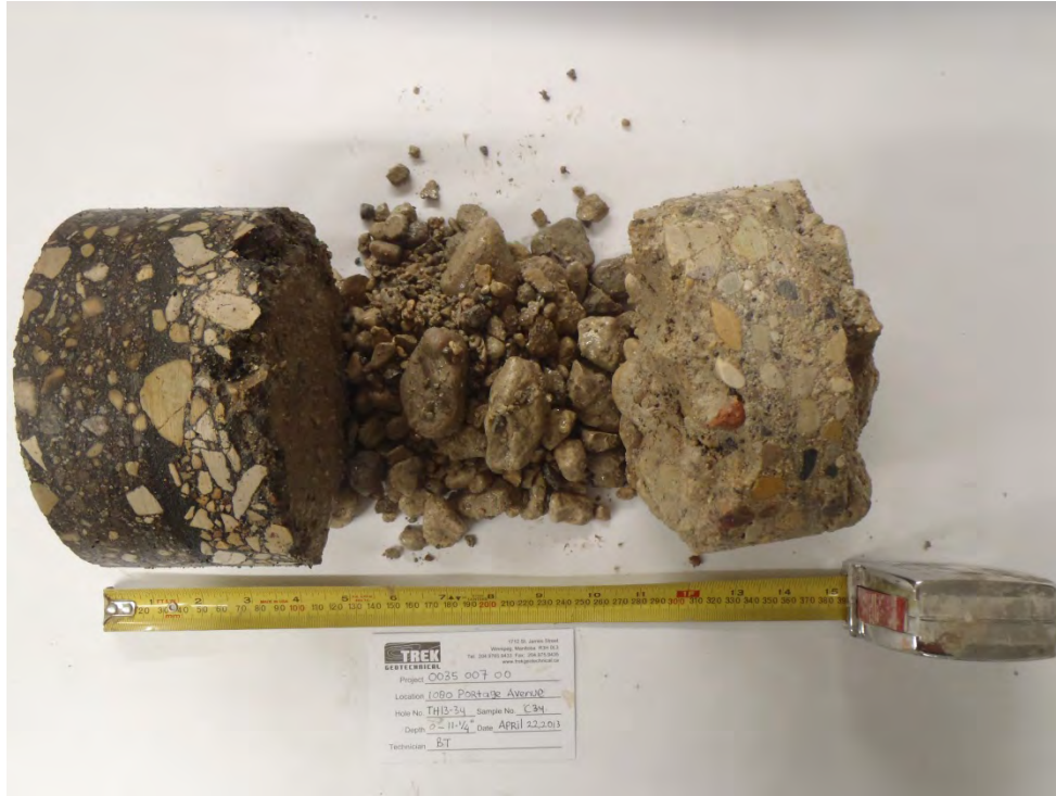
Photo 41: Asphalt and Concrete Core Sample from Test Hole TH13-34B
