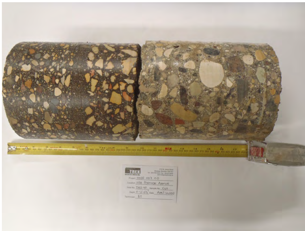
Photo 46: Asphalt and Concrete Core Sample from Test Hole TH13-40B
