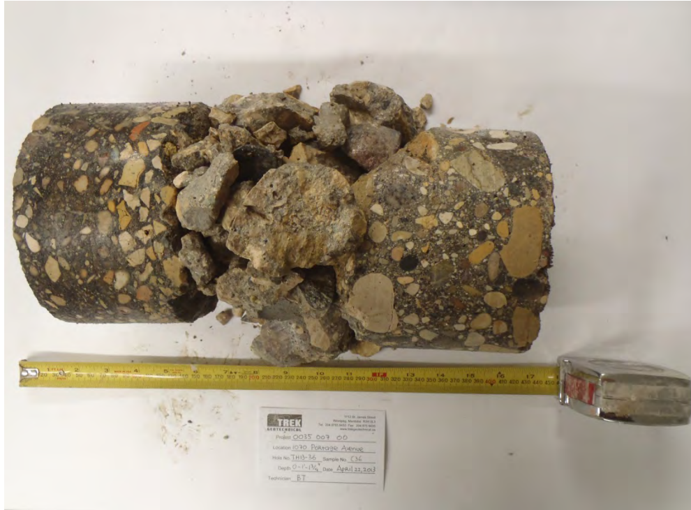
Photo 43: Asphalt and Concrete Core Sample from Test Hole TH13-36B
